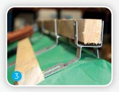
The batten holder allows easy fixing of the ridge and hip batten and is designed to withstand a wind uplift load of 800 N/m. It can be bent and split by hand to suit various heights and rafter alignment.
