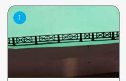
Install the sarking and battens as normal across the roof except the top two battens closest to the top. When laying the sarking ensure to leave a sufficient sag (not more than 40mm) to facilitate drainage between each roof truss.
