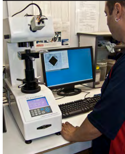
500x Magnification - Hardness Testing
